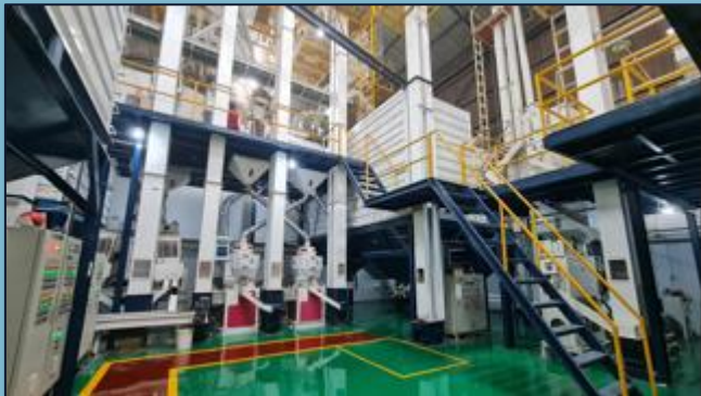
MCS Cibitung (2013), Bekasi Capacity : 5 tons/hour, 15.000 tons/year Premium Rice 1 shift, 10 hours work/day
